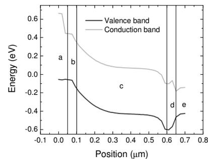
Figure 1: Energy band diagram of the integrated photodetector indicating region (a) as GaSb p-doped, (b)(c)(d) as p-i-n GaInAsSb respectively and (e) as InAsSb n-doped
