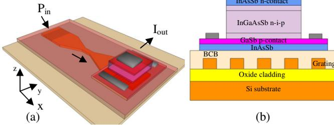
Figure 3: a) Schematic of grating-assisted design b) cross section in x direction
