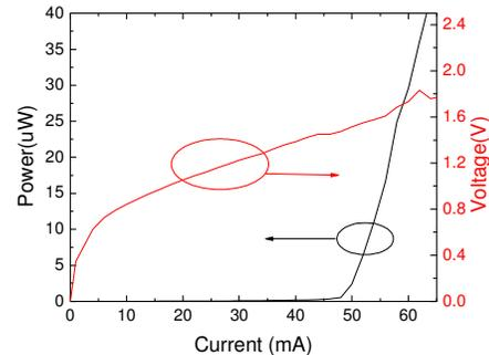
Figure 8: LIV characteristic of the laser with foot print of  $15\mu\text{m} \times 490\mu\text{m}$
