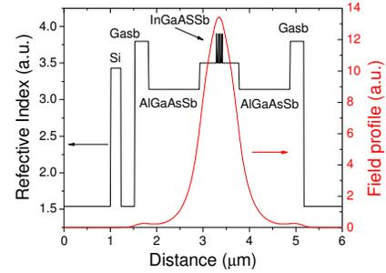
Figure 4: Refractive index profile of the laser epitaxy and laser mode profile
