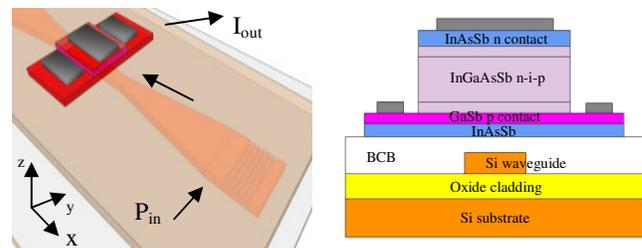
Figure 2: a) schematic of the evanescent coupling scheme b) cross section in y direction of the integrated detector
