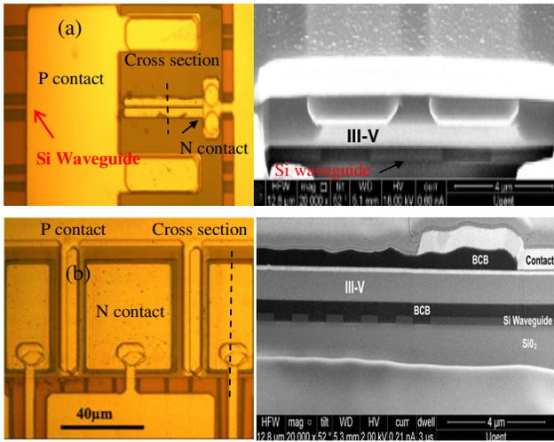
Figure 5: a) optical image (left) and SEM image (right) of evanescent coupling b) optical image (left) and SEM image (right) of grating-assisted coupling
