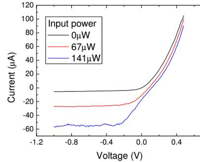
Figure 7: VI characteristic (at room temperature) for different waveguide coupled power level of the device with grating-assisted coupling design
