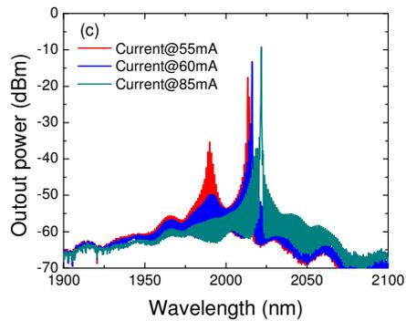
Figure 9: Spectra at different bias current
