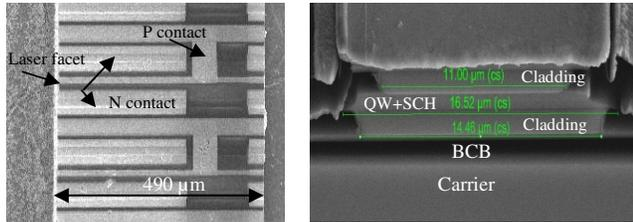
Figure 6: Image of the realized integrated laser a) top view SEM image b) SEM image of the cross section and the laser facet
