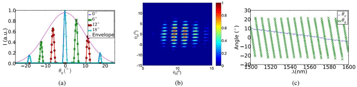
Fig. 3. (a) Measured far-field in the  $\theta_y$ -direction of a 1D OPA using thermo-optic steering at 1550 nm. The dashed line shows the envelope of the far-field pattern. (b) Measured far-field pattern of a  $2 \times 2$  OPA at a wavelength of 1550 nm. (c)  $\theta_x$  and  $\theta_y$  position of a wavelength beam steerer with an AWG of order  $q = -150$  as a function of wavelength.
