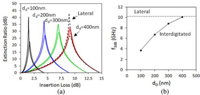
Fig. 12. (a) Calculated ER versus corresponding IL and (b) frequency response of interdigitated modulators, with variable finger width  $d_d$ .
