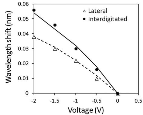
Fig. 4. Resonance wavelength shift versus voltage for interdigitated and lateral diode designs. The symbols are experimental data, while the lines show the modeled results.
