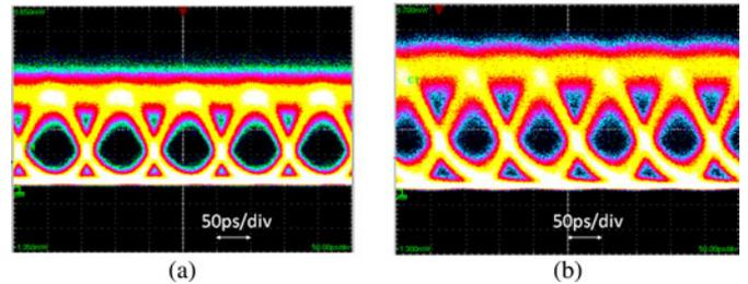
Fig. 9. Eye diagrams of (a) lateral and (b) interdigitated modulators at 10 Gb/s.
