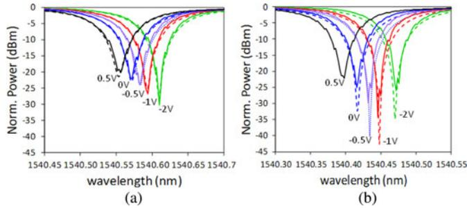
Fig. 3. Normalized transmitted power of ring modulators with (a) lateral and (b) interdigitated diode designs for voltages from 0.5 to  $-2$  V. The dashed lines show the fitted spectra.
