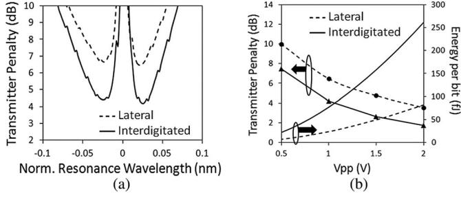
Fig. 10. (a) Expected transmitter penalty versus wavelength for lateral and interdigitated diode designs, calculated for  $1 V_{pp}$  swing. (a) Transmitter penalty and energy per bit versus  $V_{pp}$  for lateral (dashed lines) and interdigitated (solid lines) diode designs.
