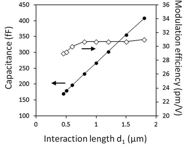
Fig. 11. Calculated junction capacitance and ME versus interaction length  $d_1$ .
