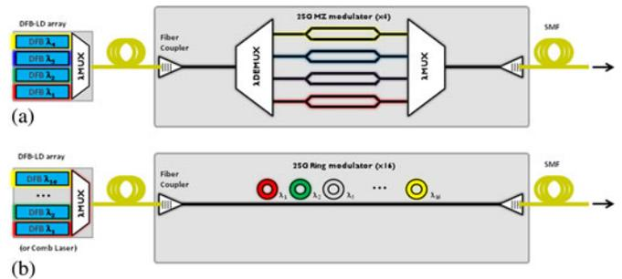
Fig. 1. (a) MZ-based silicon photonics 100G transmitter. (b) Ring-based silicon photonics 400G transmitter.
