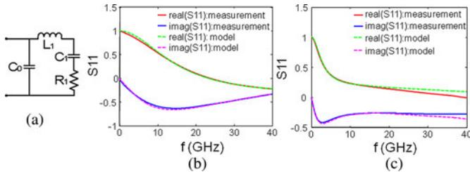
Fig. 7. (a) Circuit model and  $S_{11}$  measurements from ring modulators with (b) lateral and (c) interdigitated diode designs. The fitting to the measured data is shown by the dashed lines.
