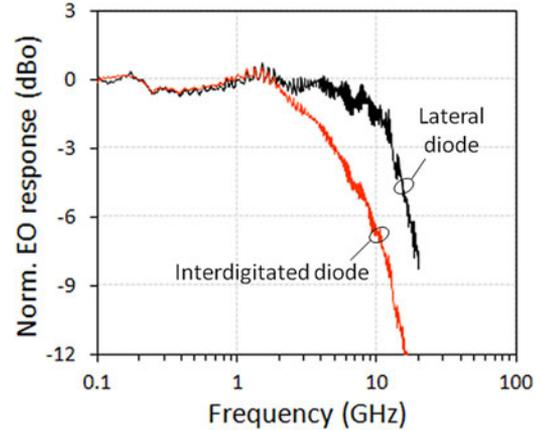
Fig. 8. Electro-optical  $S_{21}$  frequency response of ring modulators with lateral and interdigitated diode designs at 0 V bias.
