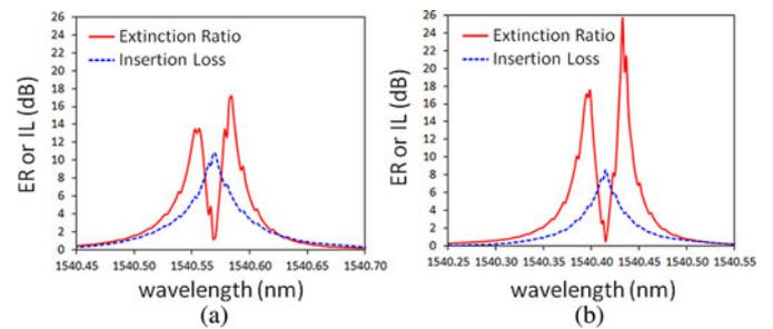
Fig. 5. Experimental ER and IL for (a) lateral and (b) interdigitated ring modulators for  $1 V_{pp}$  voltage swing with 0 V bias.
