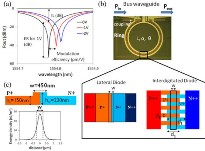
Fig. 2. (a) Typical transmission spectra of carrier depletion ring modulator for different applied bias. The ER, IL, and ME are indicated for  $1 V_{pp}$ . (b) Ring modulator schematic showing the lateral and interdigitated diode designs. (c) Ring waveguide cross section and mode distribution.
