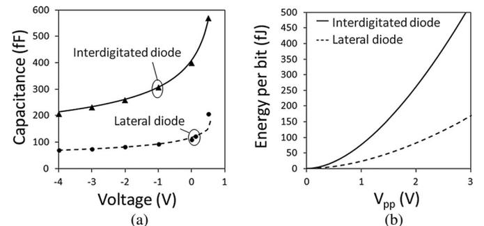
Fig. 6. (a) Capacitance–voltage measurements (symbols) and fitting (lines), and (b) energy per bit versus peak-to-peak voltage ( $V_{pp}$ ) for lateral and interdigitated diode designs.
