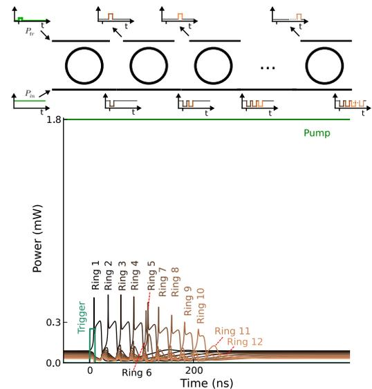
Fig. 1. (top) By cascading a number of excitable add-drop ring resonators on a common bus waveguide, a tapped delay line can be created. (bottom) When pumping a chain of 12 identical rings with a 1.8 mW CW signal with a  $-16.5$  pm offset from resonance, and perturbing it with a 10 ns long and 0.25 mW strong trigger pulse, a clear output pulse is retrieved at the 10<sup>th</sup> ring with a  $\sim 200$  ns delay. Simulated using Caphe [10], [11].
