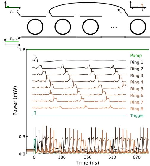
Fig. 2. (top) When feeding back the final output of a tapped optical spike delay line back to one of the inputs of the former rings, this will re-excite the chain and, consequently, an all-optical spike clock can be created. (bottom) We illustrate this for a chain of 8 rings, using the same pumping and trigger conditions as Fig. 1.
