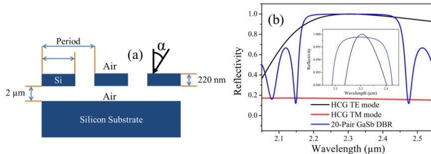
Figure 2: (a) Schematic drawing of the SOI-HCG structure, (b) reflectivity spectra of the SOI-HCG and the 20-pair GaSb-AlAsSb DBR.
