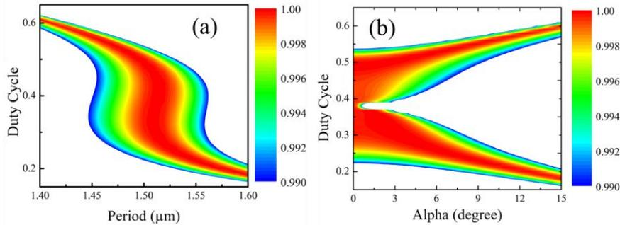
Figure 3: (a) RCWA simulated SOI-HCG reflectivity as a function of grating period and duty cycle for fixed  $\lambda = 2.3 \mu\text{m}$ , (b) contour plot of reflectivity versus duty cycle and incident angle.
