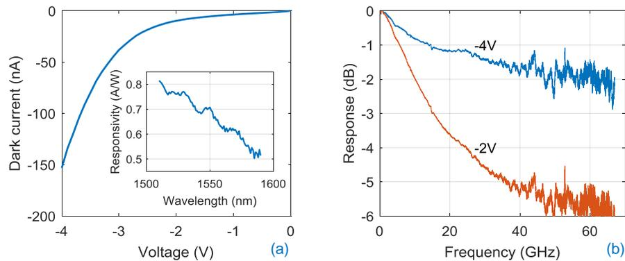
Fig. 2. (a) Measured dark current of a  $3 \times 10 \mu\text{m}^2$  PD; the inset shows the responsivity versus wavelength measured at -4 V. (b) Frequency responses of the PD measured at -2 V and -4 V.
