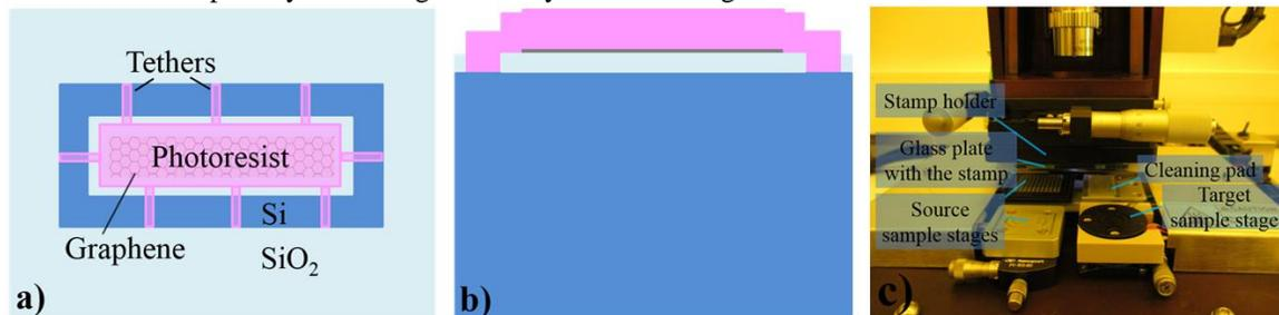
Fig. 1. The schematic of a graphene coupon on the source sample. a) Top view. b) Side view. c) The transfer printer machine showing the source, target, and cleaning pads, the glass plate with the PDMS stamp (not visible) attached to the stamp holder.
