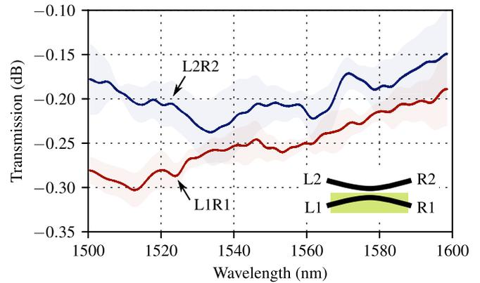
Fig. 5. Bar-port transmission of the LCC in the bar state with light going through the shielded waveguide (in blue) and through the waveguide exposed to the liquid HPC (in red).
