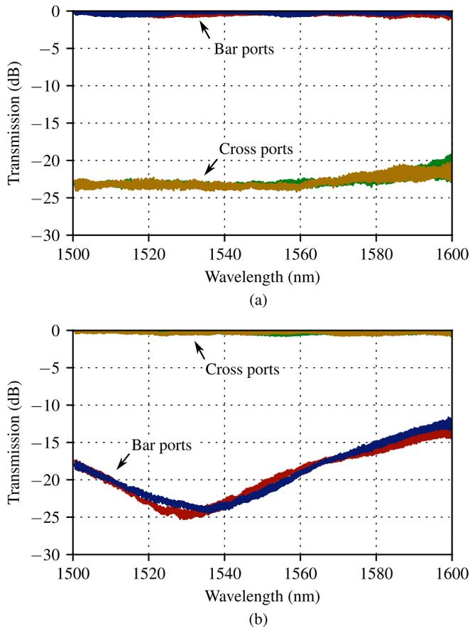
Fig. 4. Transmission of an 820- $\mu\text{m}$ -long LCC in (a) the bar state and (b) the cross state.
