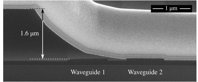
Fig. 3. Cross-section SEM image at the center of an LCC.
