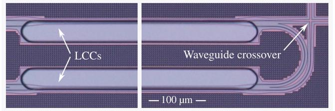
Fig. 2. Optical microscope image of a diluted SE with two LCCs.
