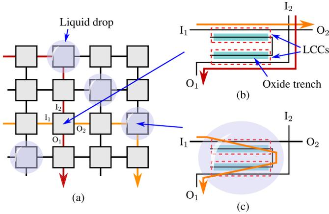
Fig. 1. Schematic of (a) a cross-bar switch circuit with diluted SEs in (b) the bar state and (c) the cross state and with indication of two light paths.
