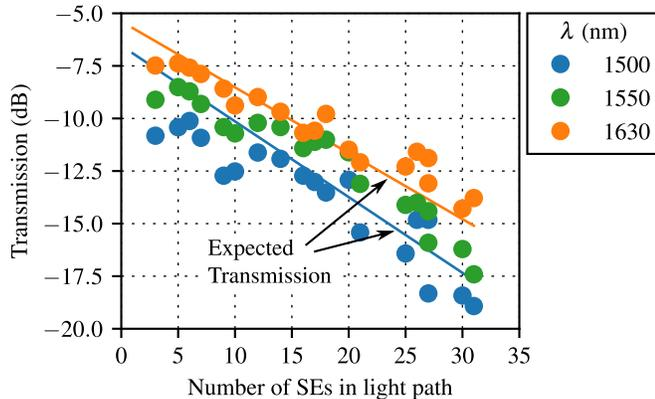
Fig. 6. Transmission of the 16 × 16 switch for different light paths and at different wavelengths. Solid lines represent the expected transmission obtained from characterized individual components.
