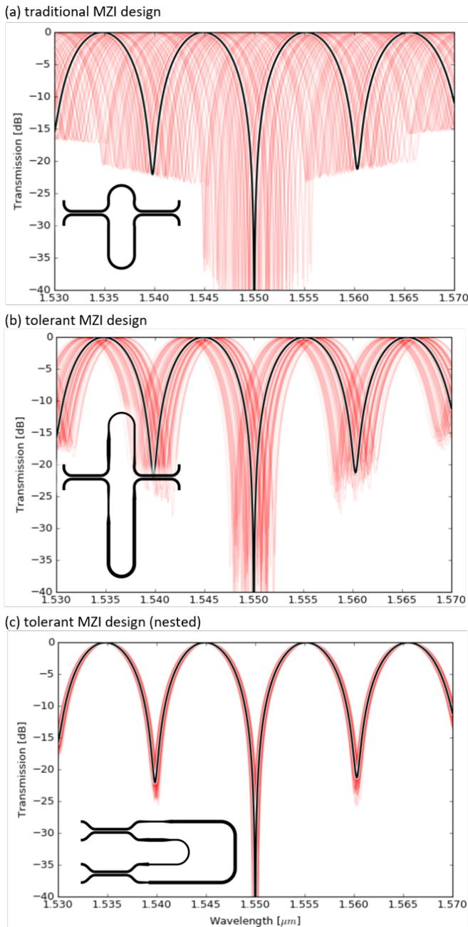
Fig. 4. Monte-Carlo transmission simulations of the MZI circuits in Fig. 3. (a) the non-tolerant design experiences large wavelength shifts, (b) the tolerant design with opposite waveguides compensates global variations, while (c) the nested waveguides make the design less sensitive to local variations.
