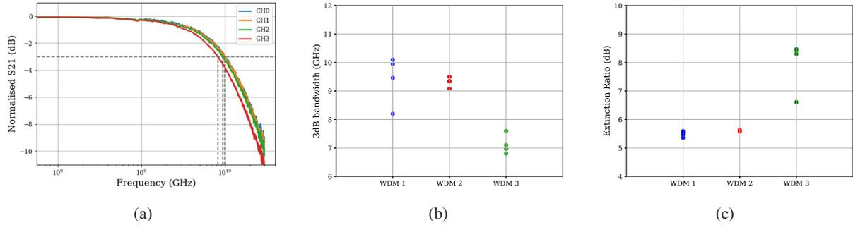
Fig. 3: (a)  $S_{21}$  frequency response measured at 0 V DC bias on a 4-channel WDM with a 500nm-wide waveguide and 100 $\mu$ m-long devices. (b) 3dB bandwidth at 0 V of the 4 channels of the three WDM transmitters. (c) Extinction ratio of the 4 channels of the three WDM transmitters, measured with 8 V voltage sweep.
