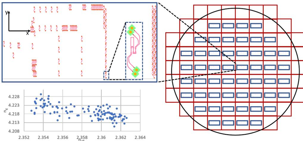
Figure 2. (a) Locations of the two-stage MZI on a die. (b) Extracted  $n_{eff}$  and corresponding  $n_g$  of die ( $X=0, Y=0$ ) (in the center of the wafer). (c) Locations of dies on the wafer. Red grid indicates dies on the wafer. The black circle is the boundary of the wafer.
