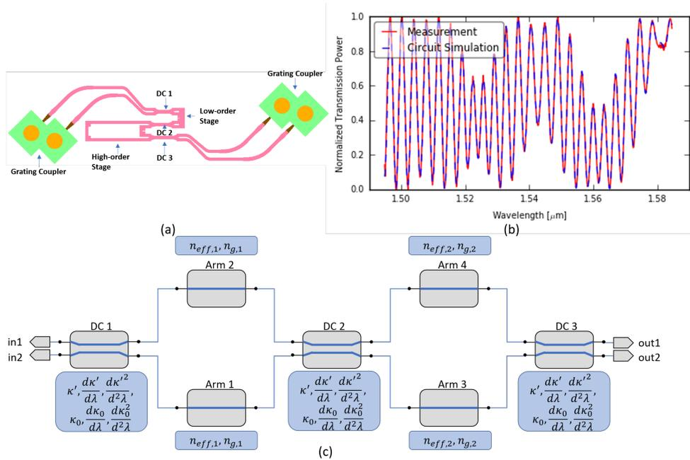
Figure 1. (a) The layout of the two-stage MZI. (b) The measured spectrum of a two-stage MZI. (c) The circuit model of the device. Two MZI stage have different  $n_{eff}$  and  $n_g$  led by the local process variation.
