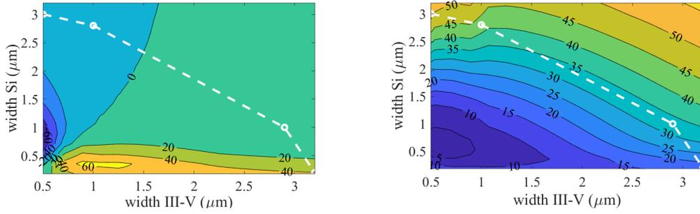
Figure 2. (Left) Calculated values of  $\gamma$  for several waveguide width combinations of III-V and Si, (Right) Calculated values of  $\kappa$  in  $mm^{-1}$
