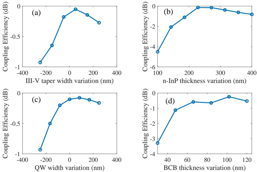
Figure 4. Effect on coupling efficiency with 1  $\mu\text{m}$  misaligned III-V and Si taper of (a) III-V taper width variation, (b) n-InP thickness variation, (c) QW width variation, and (d) BCB thickness variation
