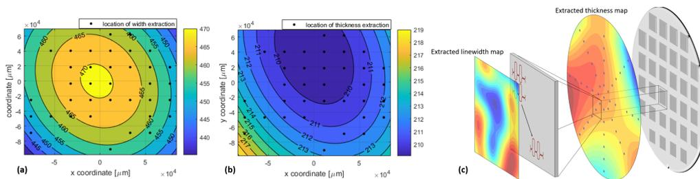
Fig. 2. Extracted wafer maps for the (a) width and (b) thickness. Layout-aware yield prediction is performed using the Monte-Carlo simulations based on the extracted width and thickness maps shown in (a) and (b).
