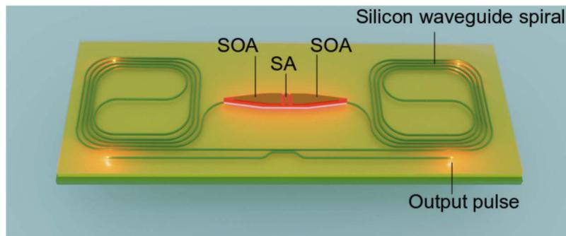
**Fig. 1.** Layout of the hybrid 8 GHz ring frequency comb laser. Semiconductor Optical Amplifier (SOA) and Saturable Absorber (SA) are integrated within the active Indium Phosphide (InP) material. The long spiral waveguide is etched in the underlying Si membrane that is bonded to InP. Light is evanescently coupled between active and passive layers.
