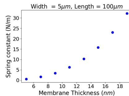
**Thickness dependence :** for fixed membrane width and length.
