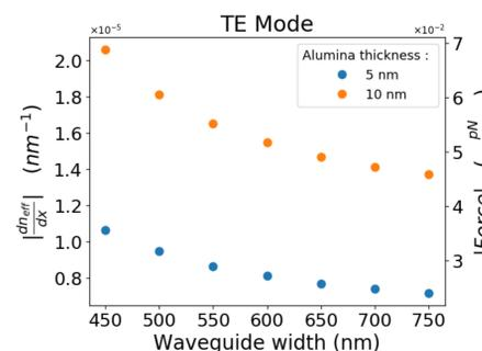
**Force dependence waveguide width :** for different thickness
