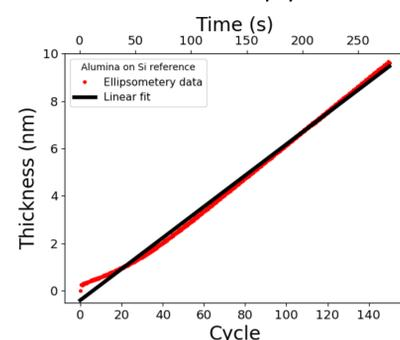
Thickness vs ALD cycles and deposition time for alumina on blank Si substrate.
