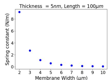
**Width dependence :** for fixed membrane thickness and length.
