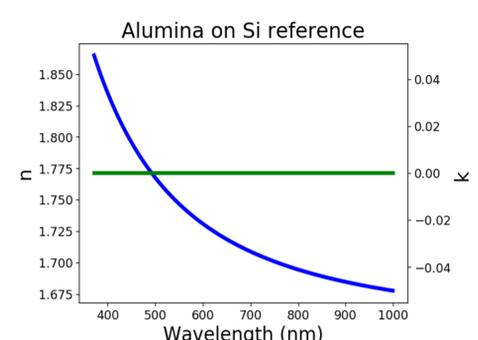
Real and imaginary part of refractive index of alumina on Si.
