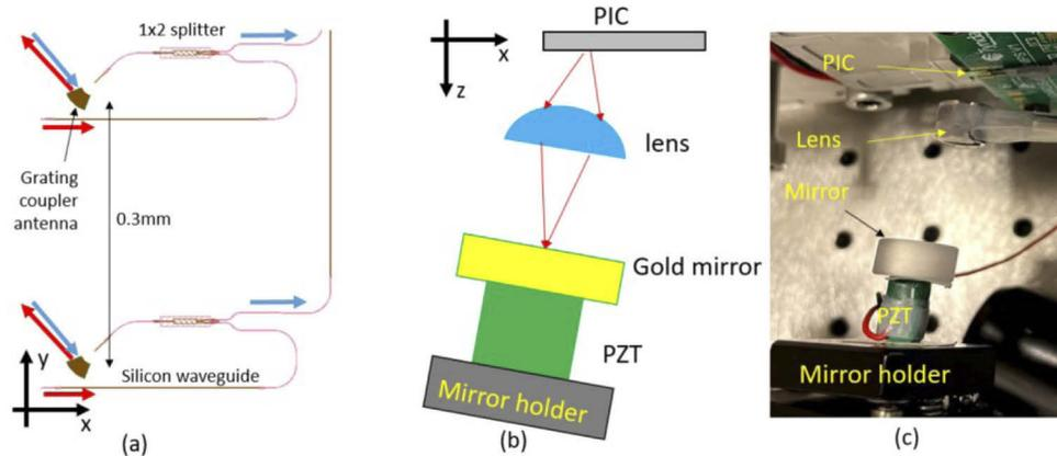
**Fig. 10.** (a) The antennas of the dual LDV design, red curves stand for outgoing light and blue curves stand for reflection light. (b) Schematic of the measurement setup to show the second-order ghost reflection. (c) A picture of the measurement setup.
