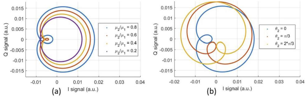
**Fig. 3.** Plots of the IQ curves based on the Eq. (1). (a) The IQ curves of LDV signals with a second-order ghost reflection with different strengths (b) The IQ curves of LDV signals with different phases ( $\theta_2$ ) between the main reflection and the second-order ghost reflection when  $\mu_2/\mu_1 = 0.8$ . In all plots, it is assumed that  $\mu_1 b/a = 0.01$ .
