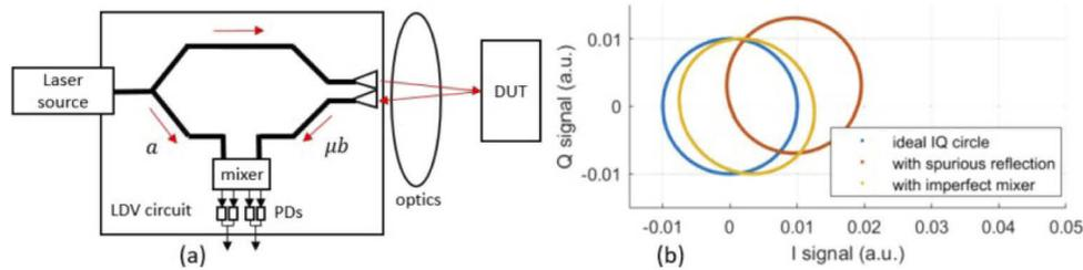
**Fig. 1.** (a). The configuration of a typical homodyne PIC LDV. (b) the Lissajous curve of I and Q signals with different distortions. Blue: no distortion; red: with DC drift; orange: with phase errors and imbalanced responsivities in PDs.
