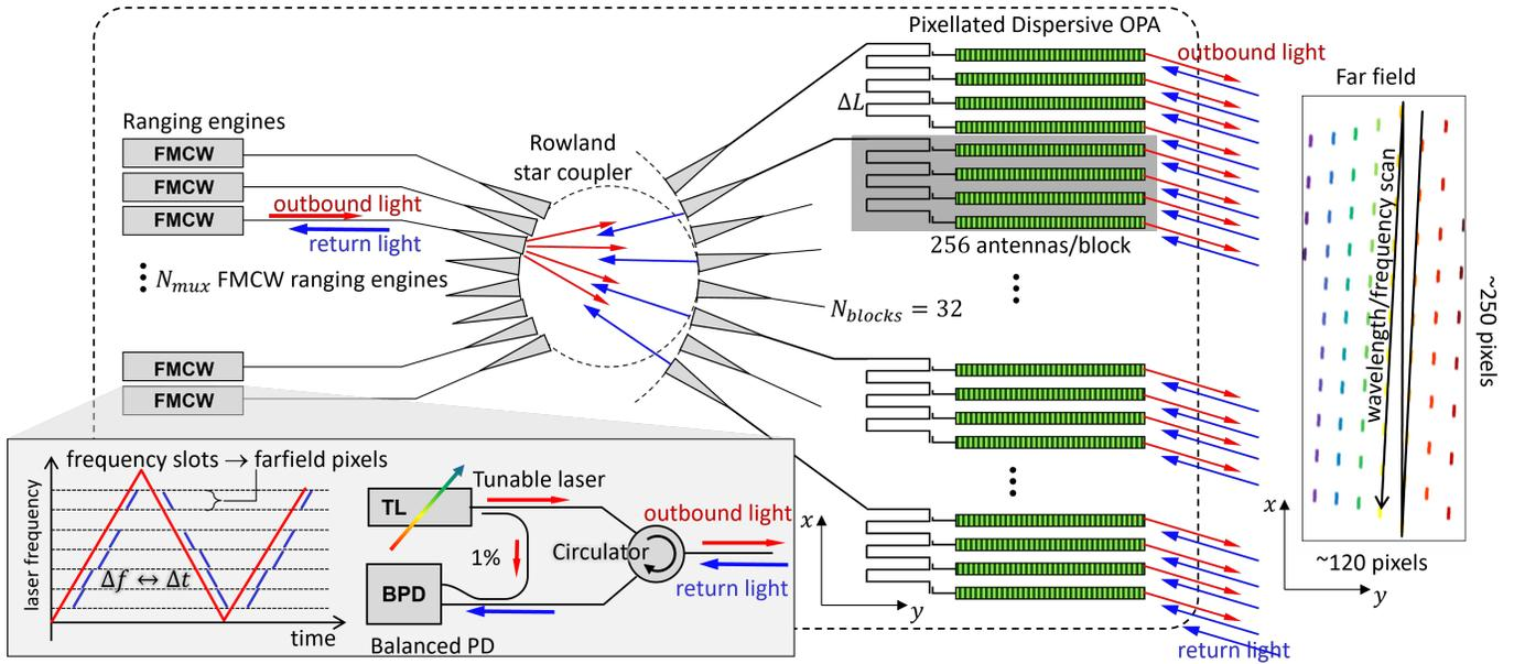
Fig. 1. Conceptual schematic of the multiplexed 2D pixellated dispersive OPA beam scanner with an FMCW ranging engine.
