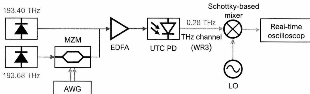
**Figure 2.** The photomixing experiment consists centrally of the optically and electrically probed PIC containing the UTC PD.
