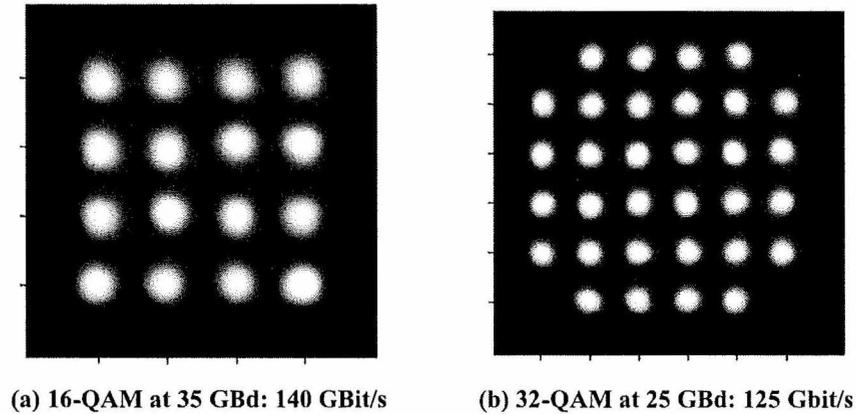
Figure 3. Constellation diagrams for both configurations show a low EVM.
