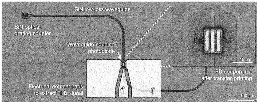
**Figure 1.** The SiN PIC consists of an optical grating coupler, SiN waveguide and electrical contact pads to probe the waveguide-coupled UTC PD.
